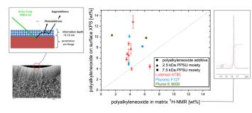
PPSU additives agglomerate on the membrane separation layer of PPSU single bore membranes
